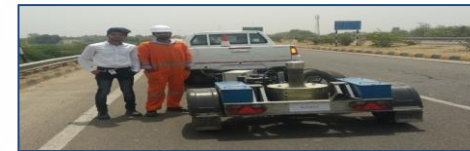
Pavement Investigation using Falling Weight Deflectometer
