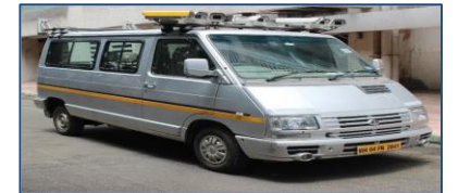
Pavement Investigation using Network Survey Vehicle
